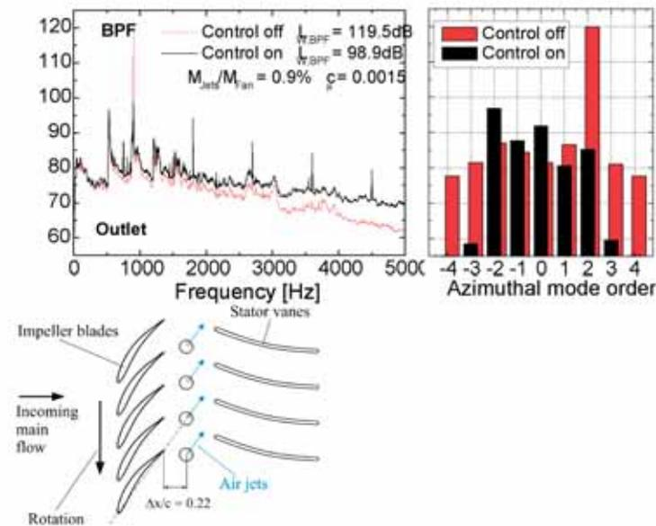
Fig. 6: Sound power spectra in the outlet duct with steady air jets (left) and azimuthal mode spectra (middle) at the blade passing frequency; nozzles placed  $\Delta x/c = 0.22$  downstream of the impeller blade trailing edges blowing in direction of the chord of the impeller blades;  $n = 3000$  rpm,  $Z = 18$ ,  $V = 16$ ,  $Z_{noz} = 16$ ,  $\varphi = \varphi_{opt}$ ; (right) sketch of the principal arrangement for this measurement.
