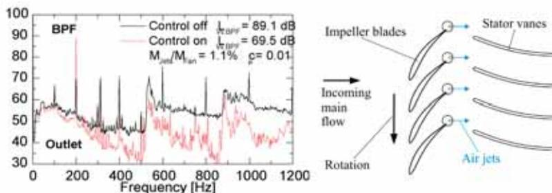
Fig. 4: Sound power spectra in the outlet duct with unsteady air jets synchronized with BPF; nozzles placed at the impeller blade trailing edges ( $\Delta x/c = 0$ ) blowing in the direction of the mean flow;  $n = 750$  rpm,  $Z = 16$ ,  $V = 16$ ,  $Z_{noz} = 16$ ,  $\varphi = \varphi_{opt}$ .
