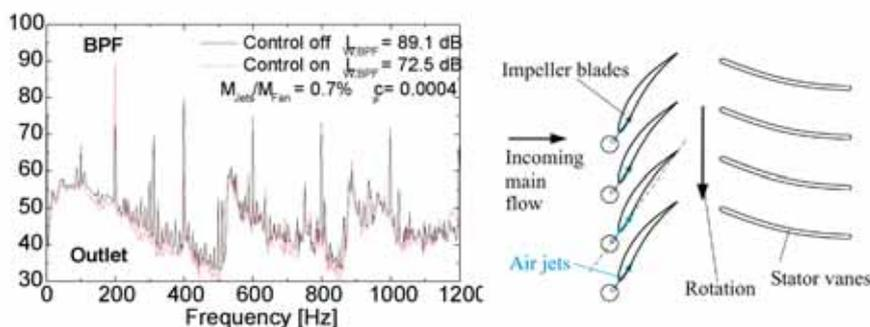
Fig. 5: Sound power spectra in the outlet duct with unsteady air jets synchronized with BPF; nozzles placed 0.5 mm upstream of the impeller blade leading edges ( $\Delta x/c = -0.009$ ) blowing in the direction of the chord of the impeller blades.  $n = 750$  rpm,  $Z = 16$ ,  $V = 16$ ,  $Z_{noz} = 16$ ,  $\varphi = \varphi_{opt}$ .
