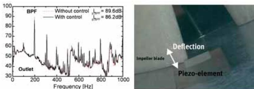
Fig. 8: Sound power spectra in the outlet duct with wall flush mounted piezo-elements (refer to Figure 3b) 0.5 mm upstream of the rotor blade leading edge, synchronized with the blade passing frequency, maximal deflection 1.2 mm;  $n = 750$  rpm,  $Z = 16$ ;  $V = 16$ ;  $Z_{\text{piezo}} = 16$ ,  $\varphi = \varphi_{\text{opt}}$ .
