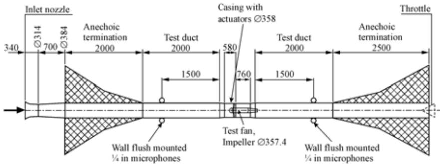
Fig. 2: Experimental set-up for the active noise control (dimensions in mm)
