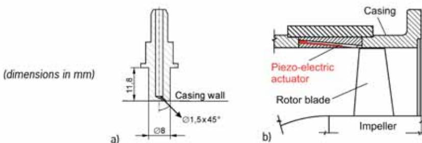
Fig. 3: a) Schematic of the nozzles used to generate the flow disturbances; b) Flow distortion with piezo-electric actuators upstream of the impeller, wall flush mounted with radial deflection
