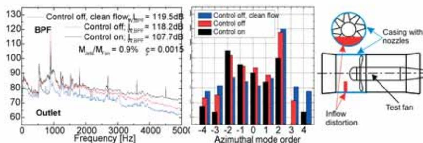
Fig. 7: Sound power spectra in the outlet duct with steady air jets (left) and azimuthal mode spectra (middle) at the blade passing frequency. Test conditions as shown in Figure 6, but here with strong distortion of the incoming flow, as depicted in the sketch (right).
