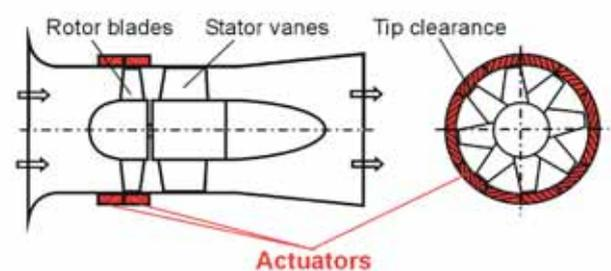
Fig. 1: Principle of the experimental set-up with actuators
